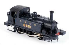
249 A metal kit-built 0-gauge 0-6-2 locomotive, 9564 in LNER black livery, two rail electric.
