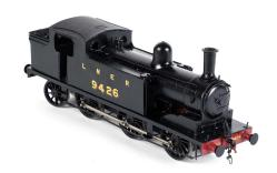
A metal kit-built 0-gauge 2-4-2 tank locomotive, 7099 in LNER black livery, two rail electric.
