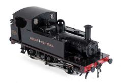
247 A metal kit-built 0-gauge 2-2-4 tank locomotive, 957 in NE green livery, two rail electric. Provenance - From the collection of Frederick William
