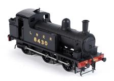
A metal kit-built 0-gauge 0-4-2 locomotive, Z5 Class 8192 in LNER black livery, two rail electric.
