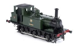
A metal kit-built 0-gauge 4-4-4 locomotive, 2143 in North-Eastern green livery, two rail electric.
