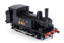
59 **A metal kit-built 0-gauge 0-6-0 locomotive,** 8430 in LNER black livery, two rail electric.
