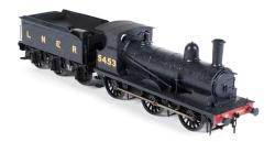
235 A metal kit-built 0-gauge 0-6-0 locomotive and six-wheel tender, 1001 in NER black livery, two rail electric.
