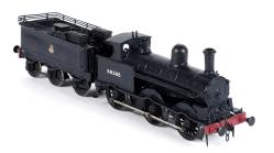
198 A metal kit-built 0-gauge 0-6-0 locomotive, 8723 in LNER black livery, two rail electric.
