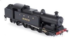
A metal kit-built 0-gauge 4-4-2 locomotive, 7500 in LNER black livery, two rail electric, probably by Ace Products.
