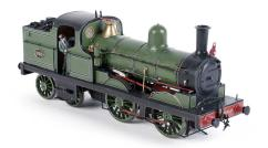
A Gladiator Models metal kit-built 0-gauge 4-4-0 locomotive and six-wheel tender, 9015 in British Railways black livery, two rail electric, stamped with maker and 'G.W.R. DUKEDOG' to underside.
