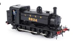
A metal kit-built 0-gauge 0-6-0 locomotive, 2012 in GWR livery, two rail electric.
